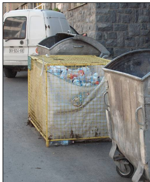
Raska municipality partly solved the problem of adapting containers to their trucks by placing large bags inside the containers. The containers are then opened, the bag is lifted out and emptied, then replaced in the container. The containers in Raska showed excellent separation and seem to be placed efficiently around the city.
